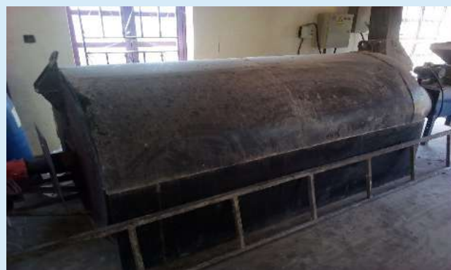
• Pic2: Flash drier that is run by electricity and diesel fuel
